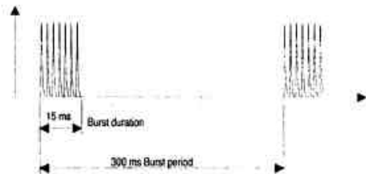
Figure 4. IEC 801-4 — Test Waveform
