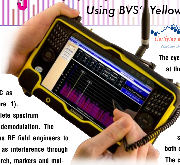
Figure 1 YellowFin WiMAX Analyzer
