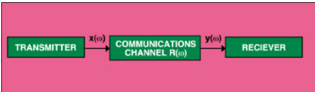
Figure 1. The Communications channel is considered to be linear and time-independent with frequency responses R(\omega) .
