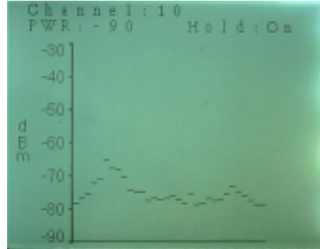
Peak Hold- 802.11 Access point
