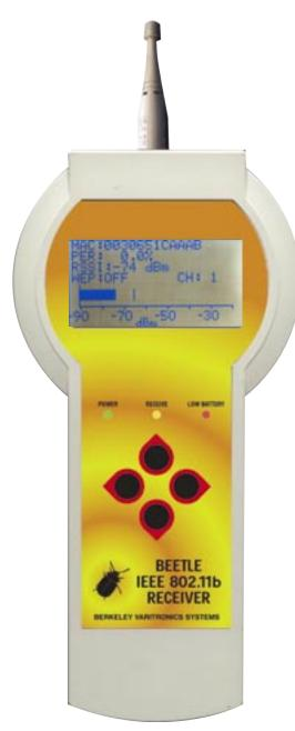
legend screen for controlling the instrument with its built-in keypad. Use the up/down arrows to scroll through menu selections. Push the right arrow button to make a selection and push the left button to move back one previous screen.
