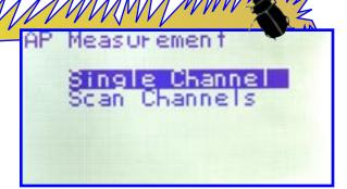
RIGHT key to choose the channel. Press the LEFT key at any time to back up to previous screen.
