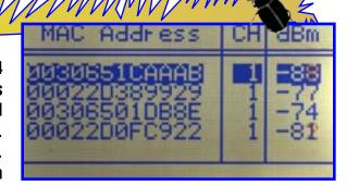
This selection clears the Beetle's memory of any list of APs that have been detected since a scan has occurred. Press the LEFT key at any time to back up to previous screen.
