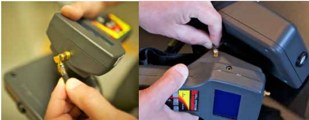
Figure 5. Attaching DF Antenna Assembly Connectors to Antenna and Laser jacks on unit (“finger-tight” only)
