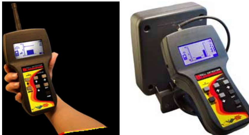
Figure 1. Bloodhound Hand-Held Unit used with the Omnidirectional or Direction Finding Antennas
