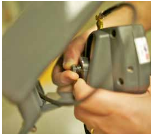
Figure 6. Securing DF Antenna Assembly Bracket to Unit with Thumb-Screw
