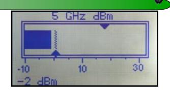
packet is detected that is above the set threshold, a bar is displayed whose length is proportional to the measured signal strength of the packet. The threshold is marked by the down arrow above the signal strength bar. This packet threshold is adjusted by pressing the UP and DOWN keys while the measurement is displayed.
