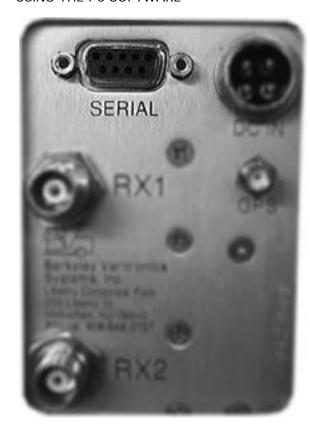
Connect the COMPANION to the PC serial port COM 1 or COM 2 using  $\,$
