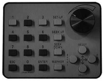
SEEK DOWN- Current Selected receiver SEEKS DOWN in frequency until a frequency is found that is >= the SEEK dBm threshold. (FREQ1 or FREQ2 must be highlighted)
