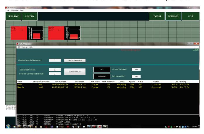
The server application also communicates to any number of client applications running on remote machines. It will pass requested information from/to the clients as well as the sensors.
