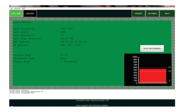
A bar graph showing the last power report is on the right-hand side. It also shows the high and low watermark readings since the last reset. Last reported threshold is also displayed in the graph.
