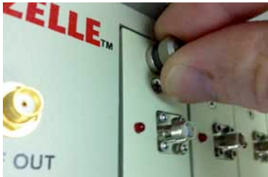
Loosen knob before removing
