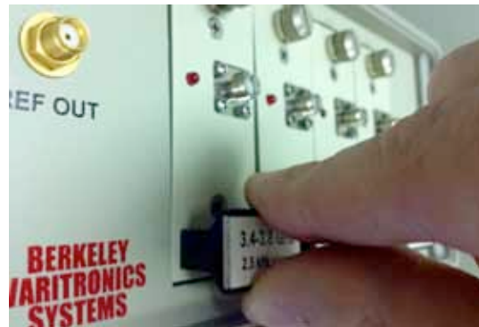
Pull on handle to remove or replace module
