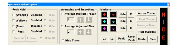
The Trace Settings dialog box allows the user to make settings and changes to the spectrum waveform such as Peak hold, Multiple and Adjacent Bin Averaging, and placing markers on the waveform.
