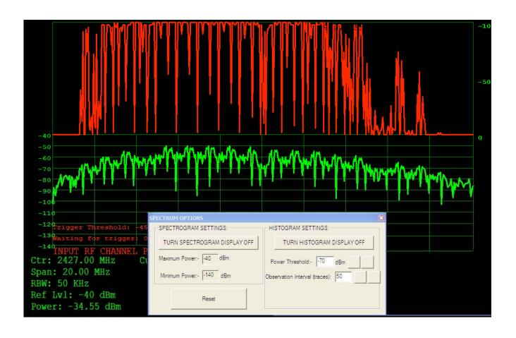
Interference Assist: The interference assist screen is a helpful tool for the user to identify difference sources of interference from the spectrum signatures. It acts as a guide for the users to identify Direct Sequence Spread Spectrum, Frequency Hopping Spread Spectrum, Continuous Wave (CW) and Bluetooth waveforms and the devices which create these waveforms.
