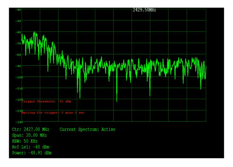
Using the Spectrum Control Dialog Box shown on the previous page, the following settings can be made:
