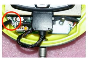
Connect the dongle hardware cable only to this PORT
