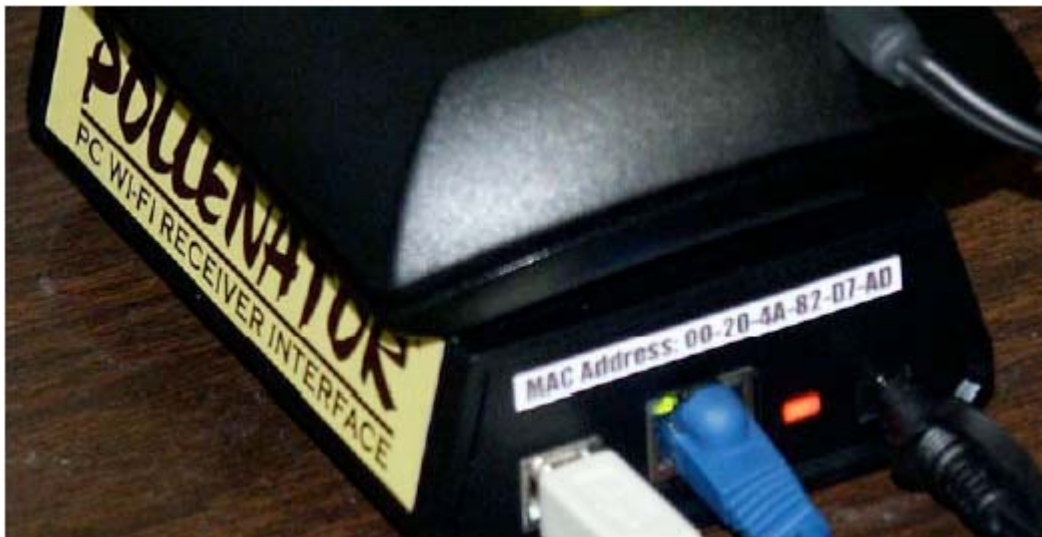
Fig 2: Ethernet/USB and the Power Supply connection on the Pollenator.
