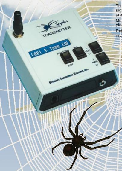
The Spyder is a self-contained frequency agile signal source for "walk-about" analysis and propagation studies.
