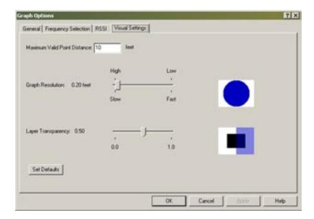
Maximum Valid Point Distance is used to determine areas of the map that have not been adequately covered by the measurement data. Such areas show up in gray on the report from a measurement point that will be considered close enough to that point to effect coverage graph. This
