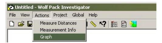
After the graph options have been selected, select Graph on the Actions menu. A dialog box will appear indicating the progress of the Investigator. If it is desired to speed up the Investigator, the Investigator resolution can be decreased in the Visual Settings of the Graph Options.
