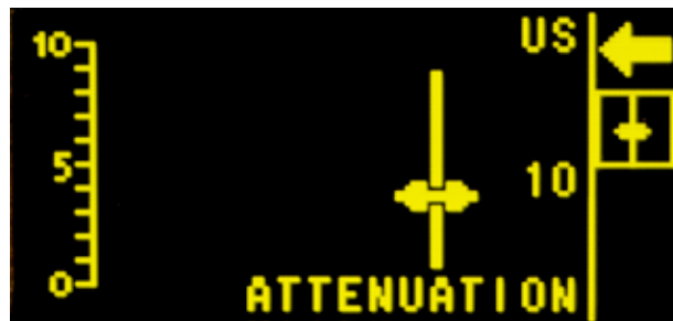
Figure 20. ATTENUATION screen (set to ~ 10dB)
