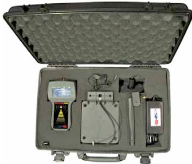
Figure 2. Wolfhound-PRO unit and accessories
