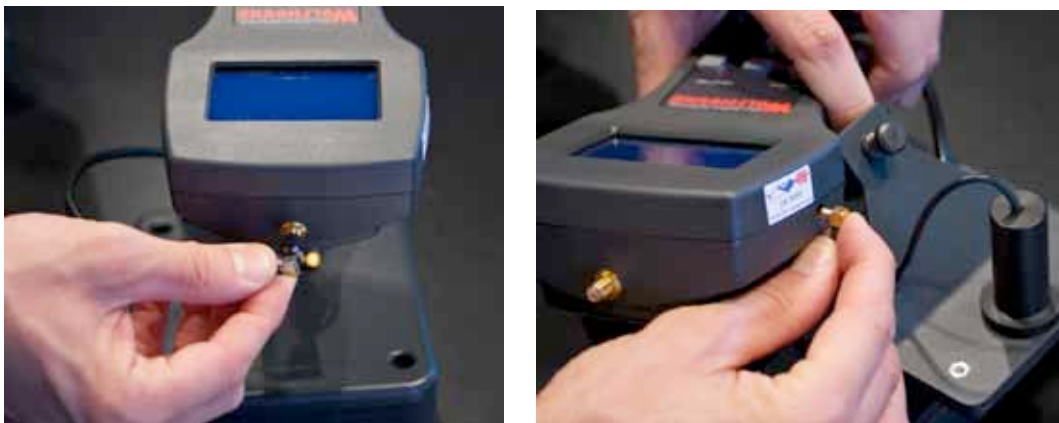
Figure 5. Attaching DF Antenna Assembly Connectors to Antenna and Laser jacks on unit (“finger-tight” only)
