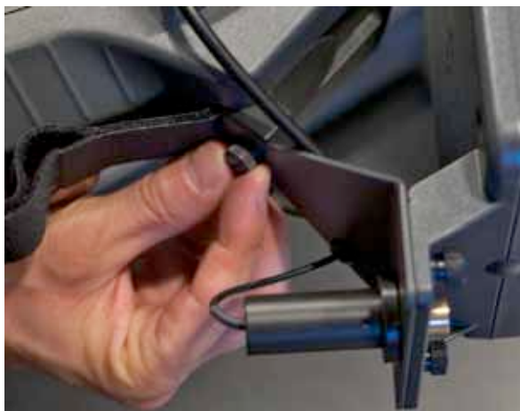
Figure 6. Securing DF Antenna Assembly Bracket to Unit with Thumb-Screw
