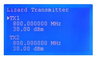
The MAIN SCREEN displays the current Dual-Band Lizard status and is also used for parameter entry. After changes are made, scroll down to Accept and press ENTER to save changes made to the TX (TX1 or TX2) shown at the top. Press ESC at anytime to leave this menu without saving any changes.
