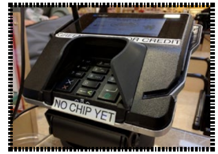
Old POS terminal only accepts mag stripe cards
