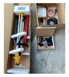
These boxes show the tripod, directional antenna, cable, vertical mounting poles and associated mounting hardware.
