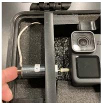
Carefully push solenoid plunger so it is back against the camera
