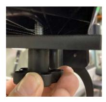
Erect the red and black poles together and connect them to the top of tripod. Feed the mount screw up through the camera box platform and tighten the camera box to the platform securely. Once you have set the camera box platform to the desired height, note the number of white tick marks to make setup easier at the next site.
