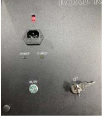
This box contains the receiver. Be sure to fully charge receiver using the supplied 110VAC power cord before operating your RoadRunner.
