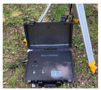
RoadRunner's cellular receiver is mounted directly into a watertight, crushproof and lockable transport case that includes an internal rechargeable battery system, touch screen and the receiver itself. The receiver case weighs approximately 15 pounds.
