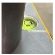
Setup the tripod on a level and stable surface. It is important to use the built in bubble level to ensure RoadRunner does not collapse due to high winds or intense ground vibrations.
