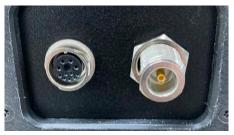
Connect the other end of the supplied cable to the RoadRunner receiver on the side of the case.
